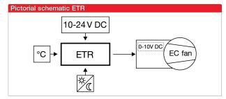
Electronic controller for differential pressure or temperature
